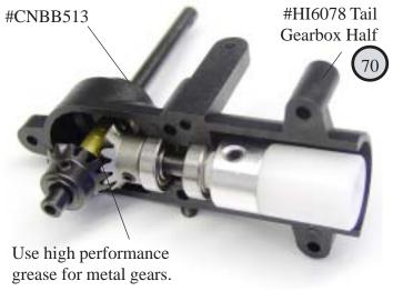
Press one M5x13 bearing into the right hand side (with mount for tail pitch lever) of the tail gearbox. Position the tail output shaft and input shaft into the gearbox half. Adjust torque fitting if necessary. Pack gears with quality grease.
