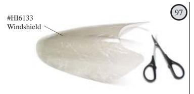
Leave the protective coating in place until after it is drilled for mounting screws. Rough cut the windshield leaving 3mm [1/8"] then carefully cut out the windshield following the line molded into the winshield.
