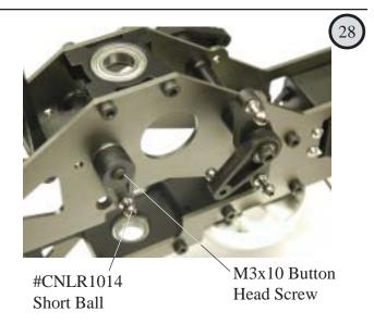
Press the rear ccpm lever onto the mount that sticks out of the right side of the upper frames with the steel ball downwards. Secure with the M3 button head screw.
