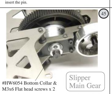
Insert the main gear assembly from the side and slide the
