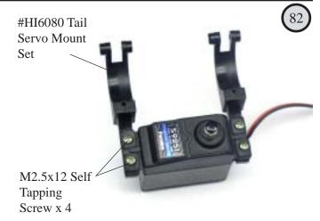
Install the rudder servo into the tail rudder servo mounts using M2.5 self tapping screws inserted through the top of the servo grommets into the vertical mounts.
