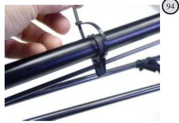
Remove the pushrod from the servo and slide through the entire range of movement. Continue adjusting the guides until the pushrod moves very smooth and then secure the tail guides with the cable ties.
