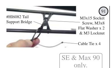
Assemble the support bridge with M3 hardware. Press each side onto the support strut and secure with the cable tie wraps provided.
