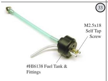
Assemble the fuel tank fittings. <u>Gently bend</u> the vent line and test until it reaches the top of the fuel tank. Order is larger outside cap, rubber stopper, smaller inside cap. Test the pickup line so it can move freely in the fuel tank.
