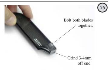
The carbon tail blades will not fit the tail rotor grips without trimming the ends. Attach the two blades together and grind 3-4mm off the end of the blades as shown.
