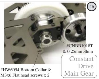
Install the main shaft thrust bearing (SE & Max only) and 0.25mm shim against the lower bearing followed by the bottom collar. Make sure the step in the collar is away from the thrust bearing. Apply locktight to the two M3 Flat head screws.
