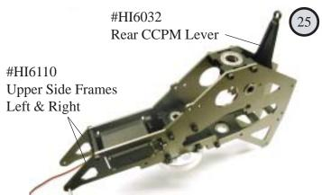
Install the rear ccpm lever into the upper frames flush with the bearing on the left side, having the mount extend out the right side frame. Assemble the upper frames <u>but do not use</u> locktight at this time.
