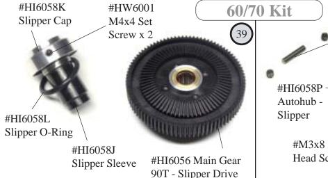
Thread the slipper cap onto the sleeve until the holes align together. Insert two M4x4 set screws at 180 degrees apart and tighten gently. Later when the main shaft pin is attached, these can be removed and locktighted in place.
