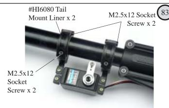
Wrap the tail mount liners around the tail boom and trim if necessary. Install the rudder servo mount assembly onto the tail boom, over the liners and secure using the M2.5 socket screws. Leave these loose until after the tail pushrod has been attached. Attach the rudder servo horn, positioning the steel ball at 12-14mm from the servo center.
