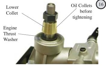
Ensure that the split in the collet is positioned away from slot for the Woodruff key. The lower collet is a tight fit to the crankshaft. Use the engine nut to start the collet onto the crankshaft, apply oil to collet.
