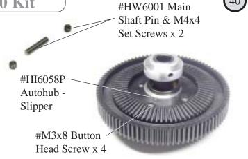
Slide the autohub for the slipper drive from the bottom of the main gear. Attach with M3 button head screws and tightening evenly. Insert the slipper cap assembly, capturing the o-ring under the cap against the autohub.
