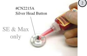
Press in the damping o-rings into the rotor head block. Lubricate with light oil. Bond the threaded stud into the head button using permanent locktight then apply more permanent locktight and bond into the top of the rotor head block.
