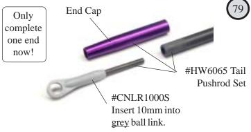
Insert the M2 threaded rod 10mm into the grey ball link. Slide the end cap over the carbon tube and make a mark, remove and sand the carbon up to this mark for better adhesion. Using JB Weld or Epoxy bond in place. Only complete one end at this time. Thread the ball link into the end cap until it stops using threadlock.
