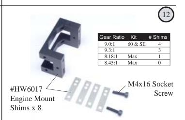
Before installing the engine, check the gear ratio to determine the correct number of shims to install between the mounting lugs on the engine and the engine mount.
