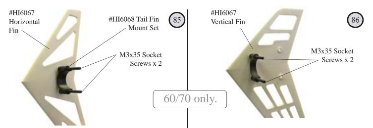
Insert the M3 socket screws through the top of the plastic fin and through the top tail fin mount (straight ends). <u>Notice that the bottom fin mount is angled for comparison.</u>
