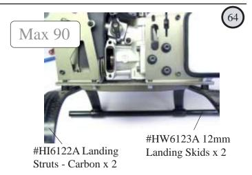
Attach the landing gear frame to the mechanics with M3x8 socket screws and locknuts. Attach the landing gear with M3x20 socket screws, M3x10 flat washers (against struts), M3x9x4 spacers and M3 locknuts, sliding the front skids into final position. Mark, scuff and bond the skids to the structs with JB Weld.
