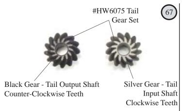
Looking down on the two tail gears notice that the black gear has teeth that are in the opposite direction to the silver gear. Make sure the black gear is mounted to the tail output shaft.
