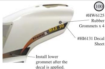
Clean the canopy. Trim the decals from the sheet and apply to the side of the canopy before the lower grommet is installed. Cut through the decal and install the lower grommet through the canopy.
