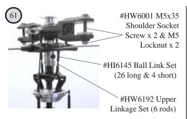
The main rotor grips will accept rotor blades that have a root thickness that is from 12mm to 18mm and have a 5mm hole. Carbon Rotortech and wooden Aerotech blades are designed for 5mm blades bolts.
