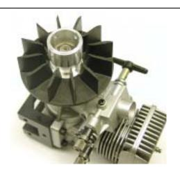
Position the fan assembly, apply oil to the collet and insert the upper split collar and the original engine nut. Clean the engine threads and apply locktight to the engine nut and tighten in place.
