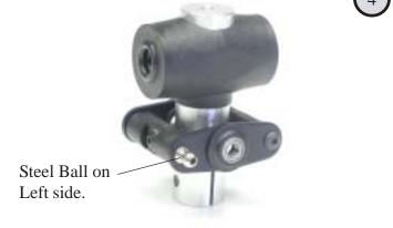
Assemble the seesaw part around the rotor head block. Bond the bearing cups to the metal offset plates.
