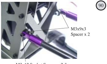
M3x12 Socket Screws x 2 & M3 Locknuts x 2
