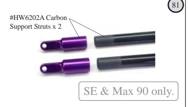
Insert and mark each end of the carbon struts where the strut fittings will overlap. Remove and sand down each carbon end until they slide easily into the fittings. Scratch inside the fittings also. Using JB Weld or Epoxy, bond the fittings in place. Make sure each strut has the fittings 90° degrees to each other.
