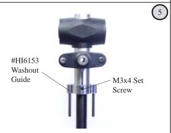
The washout guide should be positioned against the rotor head block, with the pins aligned parallel to the feathering spindle.
