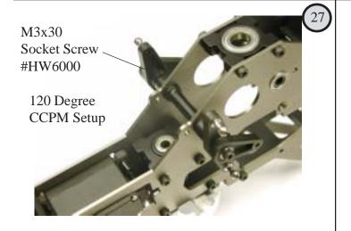
Apply locktight to the threads on the inside standoff, insert between the frames and attach the ccpm cyclic bellcranks being careful to observe the correct direction. For 140 Degree ccpm setup, move bellcranks to forward holes.
